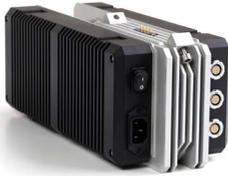
**PSU** - The brain of the operations, gives power and controls the light modules. The PSU will accept AC Voltage range of 90v-260v and will only draw 300 watts at 3 amps Max for DS3 unit.
