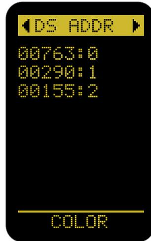
DMX addressing info is stored in the light module. This means that when switching modules between PSUs the light module will hold its address information.
